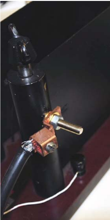
Figure 2. Current connection lug on 1 m \Omega shunt.
