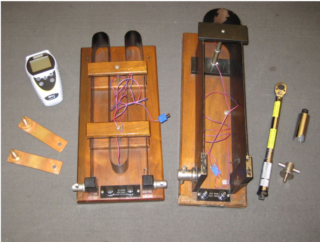
Figure 4. Artifacts for the second round of the shunt ILC.
